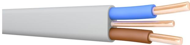
Prysmian 6242Y is a flat PVC insulated and sheathed low voltage wiring cable typically used for small power and lighting applications. Two cores with bare CPC
