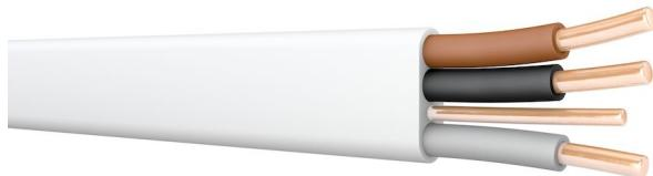
Prysmian 6243B is a flat triple core Low Smoke, Zero Halogen (LSOH®) cable designed for installation as clipped direct, on tray or in basket and also buried within plaster or embedded in walls
